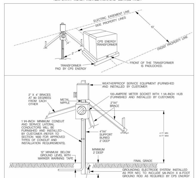
1. STANDARD INSTALLATION FOR URD TRANSFORMER AND PLACEMENT OF TML IS ON FRONT OF LOT BUT MAY BE ON REAR OF LOT
