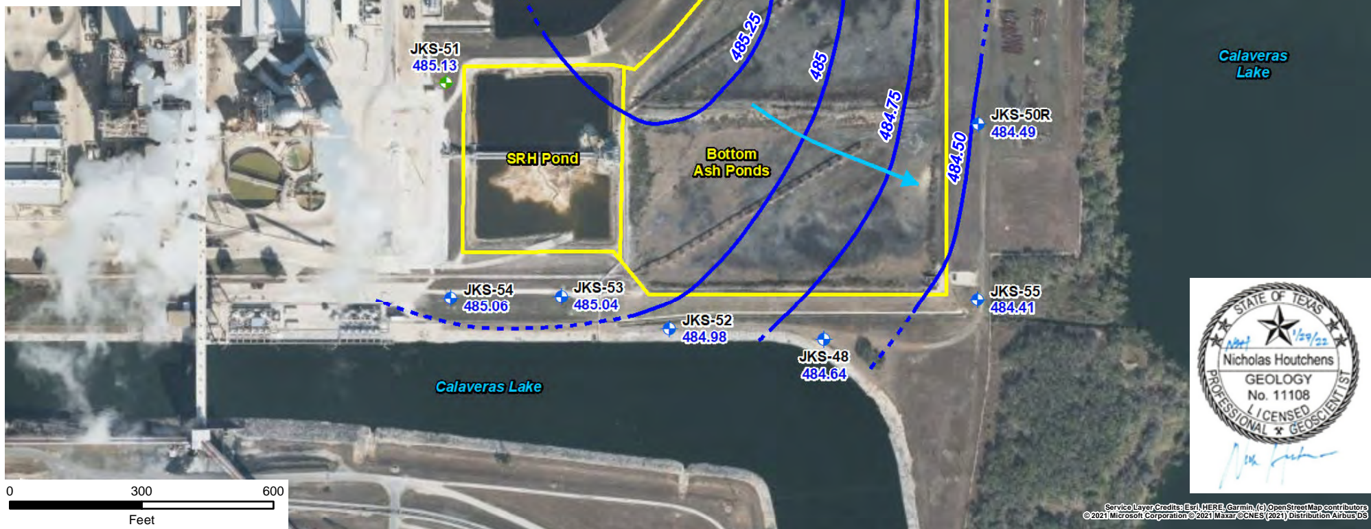
FIGURE 3A POTENTIOMETRIC SURFACE MAP - FEBRUARY 2021 Southern CCR Units CPS Energy - Calaveras Power Station San Antonio, Texas
