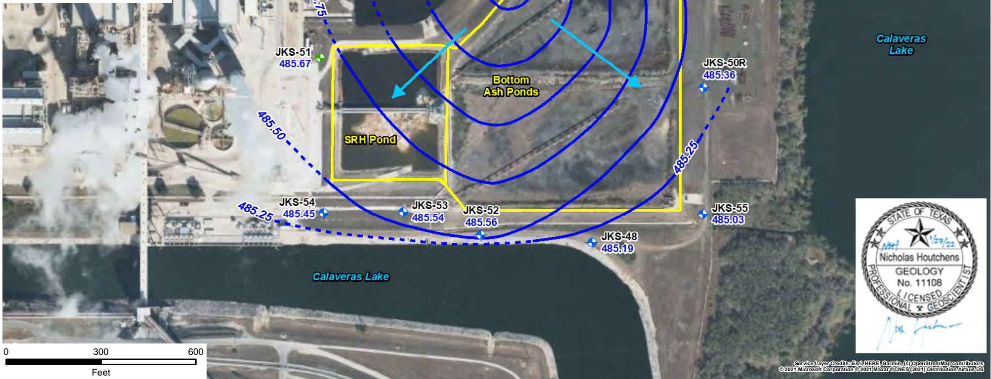
FIGURE 3D POTENTIOMETRIC SURFACE MAP - AUGUST 2021 Southern CCR Units CPS Energy - Calaveras Power Station San Antonio, Texas
