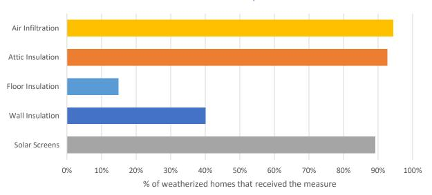
Air infiltration, attic insulation, and solar screens are the most common envelope measures.
