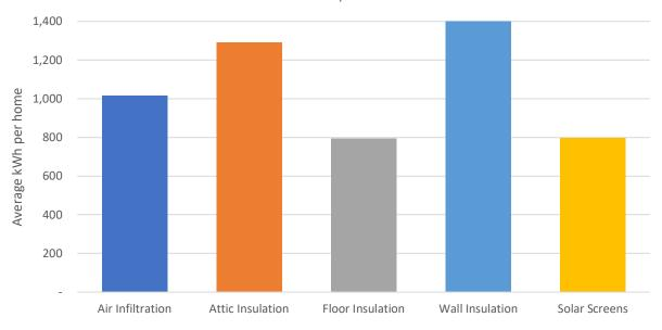
Wall and attic insulation delivered the largest average energy impacts per home for envelope measures.
