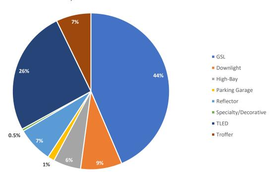
Screw-in or plug-in GSL and reflector lamps make up over 50% of desk review sample. TLEDs make up over 25%. These lamps are easier for customers to identify and install without the assistance of a contractor.
