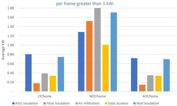
Each envelope measure produced an average NCP kW per home greater than 1 kW.
