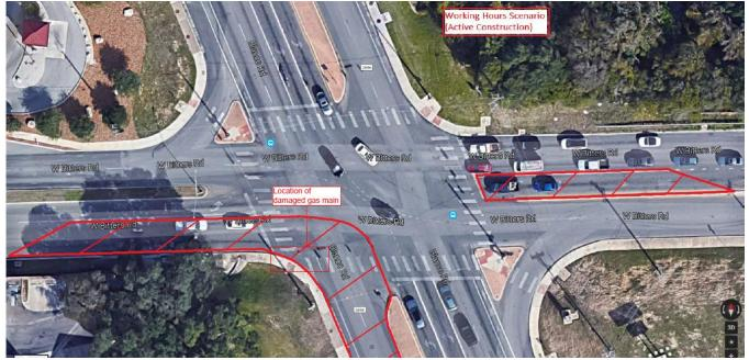
Proposed lane closures for inactive construction (non-working hours):
