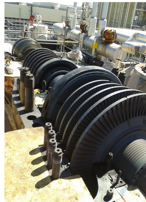
Steam Turbine Rotor During Plant Outage
